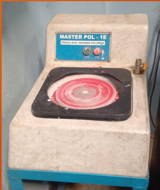
Single Disc Grinder Polisher
