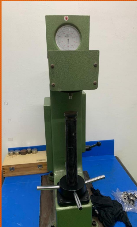
Rockwell Hardness Tester
